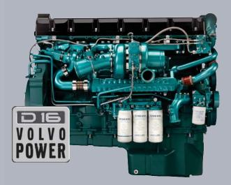
The D16 is fully EPA compliant. All regulated pollutants have been reduced 99% from untreated levels. Volvo meets these demands with outstanding reliability and economy, in part because we use Selective Catalytic Reduction for the highest efficiency. SCR allows us to pursue a passive regeneration concept that uses NOx in place of diesel fuel to regenerate the soot, further reducing your cost of operation.
