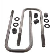
Grade 8, cold rolled Kits contain 2 bolts, 4 washers, 4 nuts Made in North America U-bolt, G8 SR, 1-1/4" x 4" x 15.5" UBK01-4015
